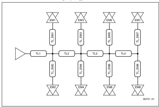
Table 12. PCI-X 66 MHz Embedded Routing Recommendations
